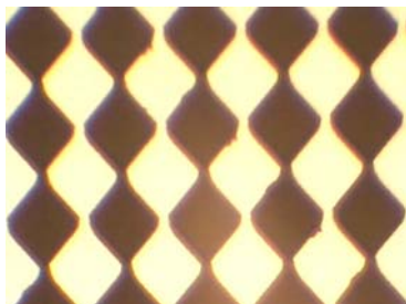
Figure 10: Squares with 16x16 pixels. It is clear that even at 16x16 pixels the image is heavily distorted.
