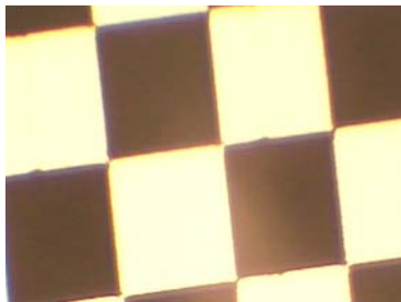
Figure 9: Squares with 32x32 pixels. This looks good even though the corners in one direction are close to not being connected already.
